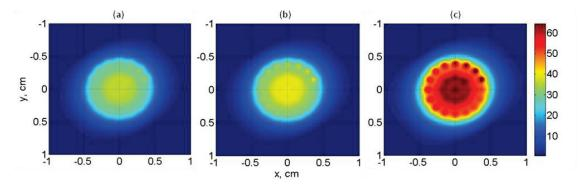
**FIGURE 4.** Temperature rise maps in the focal plane after 12 seconds of sonication for protocols with the same time-average power but different peak intensity at the array elements of 1.2 W/cm<sup>2</sup> (a), 4 W/cm<sup>2</sup> (b) and 8 W/cm<sup>2</sup> (c).
