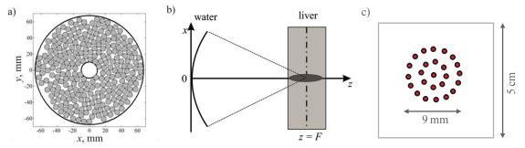
**FIGURE 1.** (a) Distribution of radiating elements on the surface of the therapeutic array; (b) geometry of the numerical experiment: ultrasound beam is focused within tissue layer (liver) centered at the geometric focus of the spherical shell (z = F); (c) Discrete trajectory of the beam's focus in the focal plane. Acoustical modeling was done both in water and in liver sample, while temperature modeling was done only in liver.
