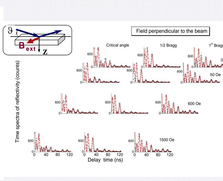
Time spectra of reflectivity as a function of the external field, measured at 3 grazing angles: at the critical one, at ½- and 1st-order Bragg maxima.
