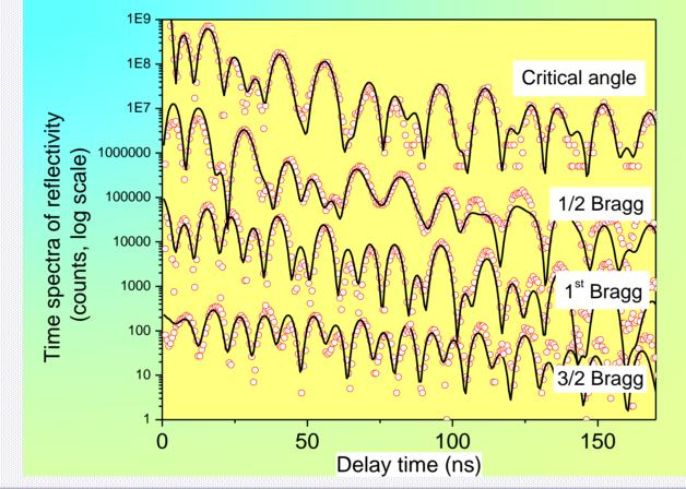
The investigated samples show the pronounced superstructure maxima (1/2 and 3/2) on the delayed reflectivity curves. That confirms the doubling of the magnetic period.
