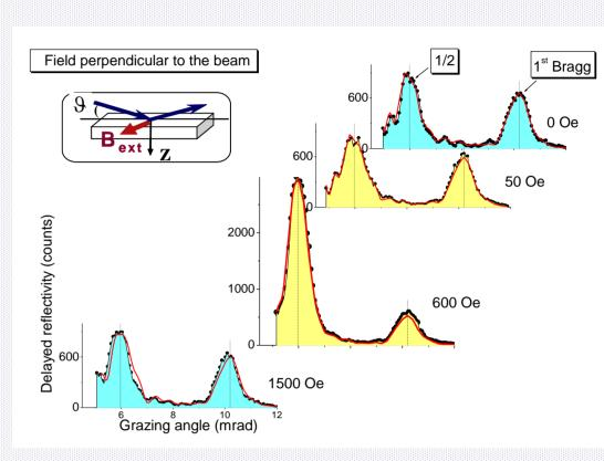
Delayed reflectivity curves as a function of the external field applied along the beam direction and perpendicular to it. The "magnetic" maximum (1/2 Bragg) essentially decreases in the longitudinal geometry at the medium field 600 Oe, but it increases at this value of the external field in transverse geometry.
