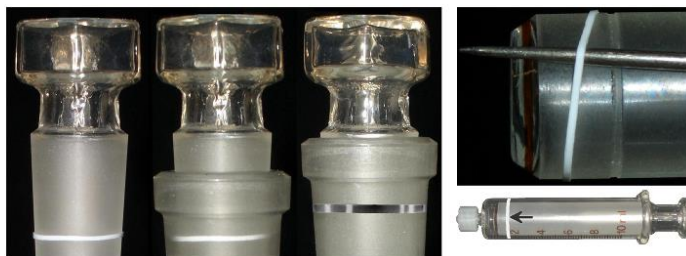
Figure 1. Left: PTFE-sealing ring fixed elastic (no groove necessary). Middle: Sealing ring intransparent without pressure. Right: Sealing ring transparent under sealing pressure. Far right: A similar PTFE ring and a piston groove make an all-glass-syringe gastight.
