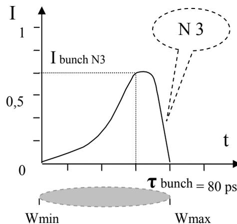
Fig. 5: A bunch № 3 up to a magnetic bunching.
