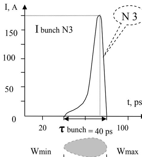
Fig. 6: A bunch № 3 after a magnetic bunching.
