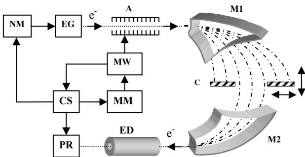
Fig. 1: A function chart of system of formation picoseconds pulses on accelerator UELV-10-10-T-1. NM - nanosecond modulator; EG - an electronic gun; A - the accelerator; M1 - a rejecting magnet; M2 - a focusing magnet; C - collimator; ED - the electro-optical detector of parameters of the beam; PR the pulse registrar; CS - the circuit of synchronization; MM - the modulator magnetron; MW - magnetron.
