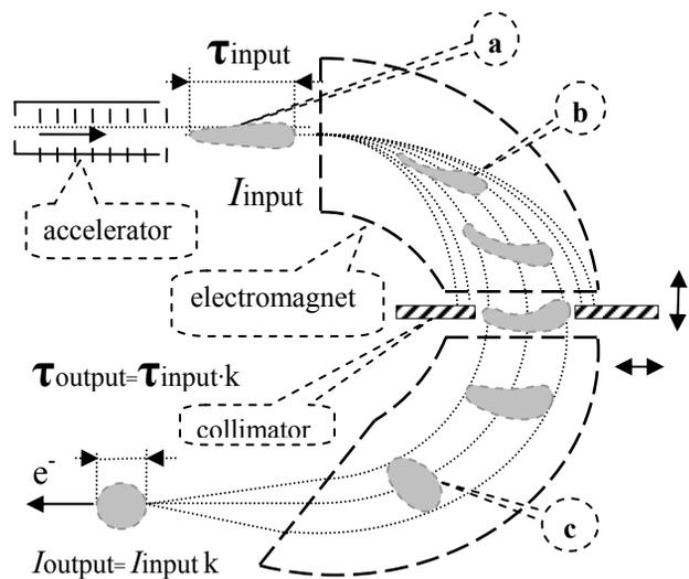
Fig. 4: Magnetic buncher and the circuit of its work: a) - intrapulse structure of the bunch; b) - a clot up to a magnetic bunching; c) - the bunch after a magnetic bunching.
