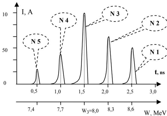
Fig. 3: Intrapulse structure of a bunch on accelerating frequency of 1886 MHz. The period of following of clots 530 ps
