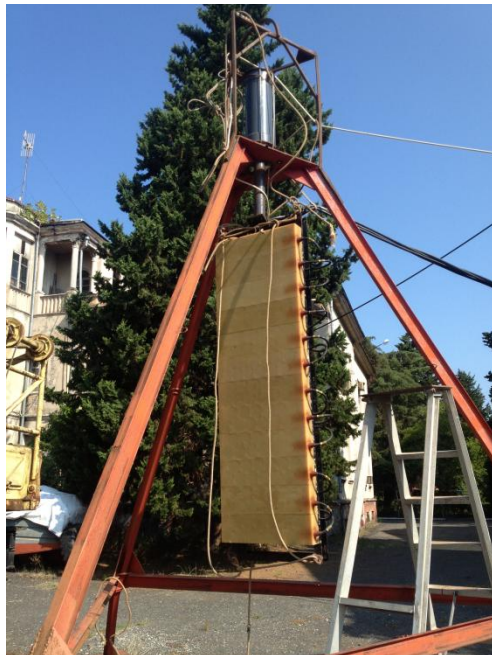
Figure 4. General view of the parametric array before installation in the sea
