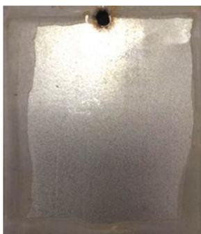
**Fig. 3.** (Color online) Photo of the zinc–polymer coating after testing for 6000 h in water (GOST 9.083-78, ISO 12944).
