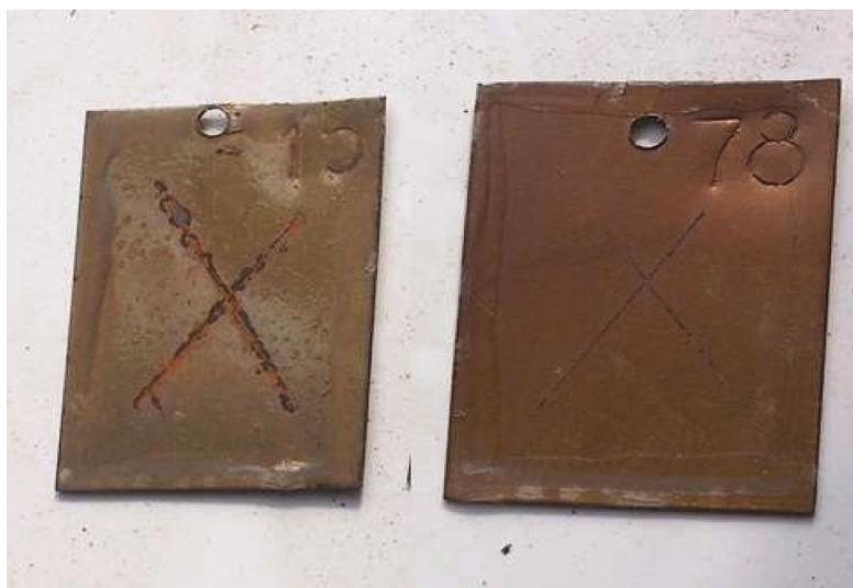
**Fig. 4.** (Color online) Photos of specimens after salt resistance testing by submerging into a 3% NaCl solution: polymer coating (left) and nickel–polymer coating (right).
