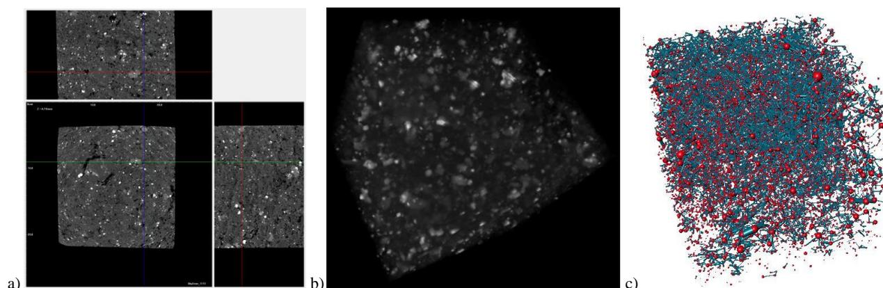
**Figure 1: Images basalt samples: a) orthogonal sections (unmodified sample HK-100-1-34); b) visualization of the location of ore minerals (shown in white) in a sample of basalt HK-102-30; c) grid model pore space of basalt sample HK-102-30 (red - pores, blue - channels)**
