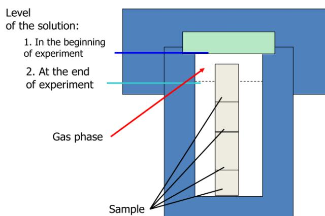
**Figure 3: Autoclave scheme**
