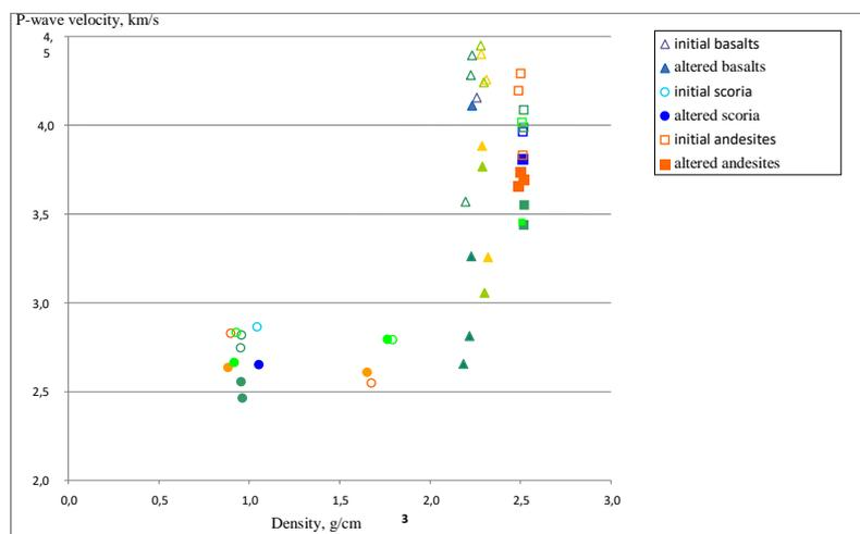
**Figure 6: The ratio of the velocity of longitudinal waves in the studied rocks and their density**
