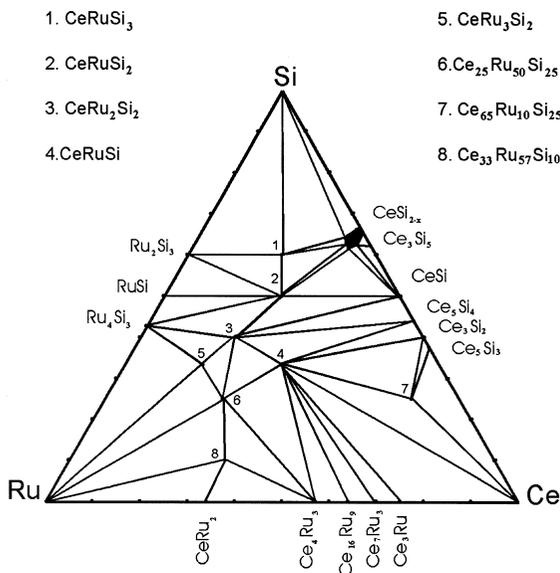
Fig. 1. Isothermal cross-section of the Ce-Ru-Si system at 600°C.
