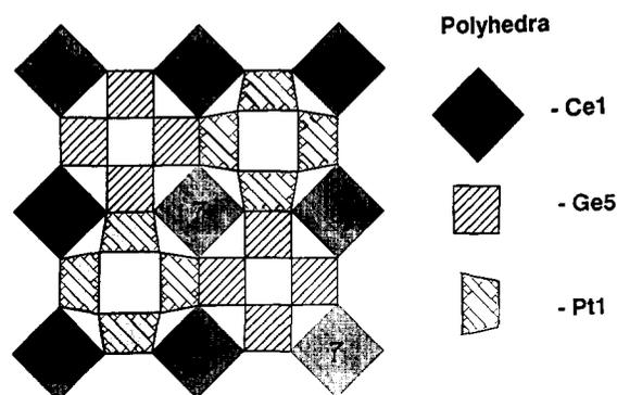
Fig. 2. Ce1, Pt1 and Ge5 coordination polyhedra packing in layer from  $Z=0.142$  to  $0.358$  (layer A).
