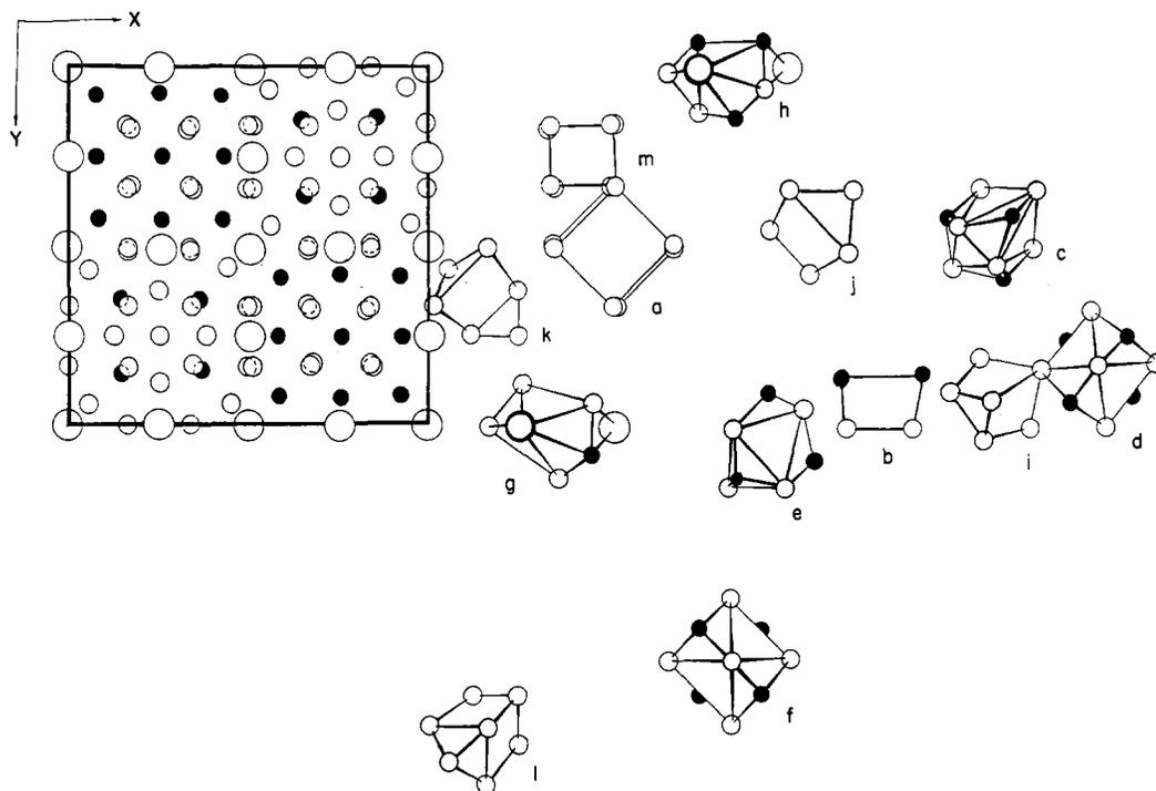
Fig. 1. Projection of  $Ce_3Pt_{23}Ge_{11}$  unit cell on to XY plane (for  $Z$  from 0 to  $\frac{1}{2}$ ) and coordination polyhedra of cerium (a), platinum (b–h) and germanium (i–m) atoms.
