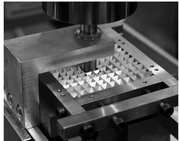
Fig. 2. Concentrated force loading of the self-locking assembly. Lateral movement of tetrahedrons is restricted by a rigid frame ('clamped boundary condition').
