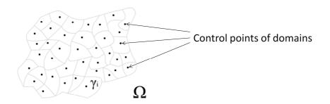
We move control points with speed  $\mathbf{u} = \mathbf{V} + \mathbf{V}_d$  and remember their circulations  $\gamma_i = \text{const } \forall i$  thus we can calculate all flow characteristics.
