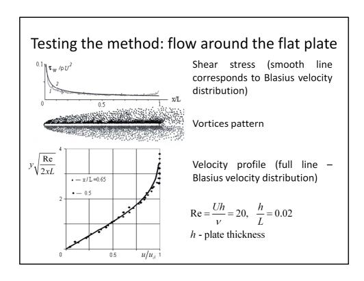
Testing of the method is shown here. This is classical problem of longitudinal flow around the flat plate at low Re number. This problem has an analytic solution.
