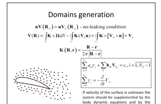
As it has already been mentioned, formation of new domains takes place on the streamlined surfaces at every time step at each node of the contour. To find circulations we use linear system, which includes:
