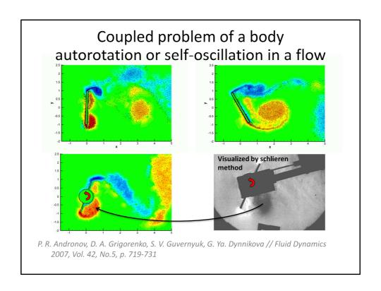
The VVD method has been used for solving coupled task of autorotation of plates and impellers around their axes. It was obtained numerically and confirmed experimentally, that, depending on initial conditions, two different regimes with autorotation and self-oscillations of the considered bodies exist. During the autorotation regime a «vortex satellite» is formed ahead of the plate moving downstream. This vortex generates lower pressure that supports autorotation.
