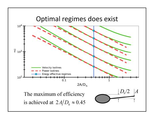
We've modeled a lot of regimes, and analyzed dependency of tadpole's velocity and power consumption on frequency and amplitude of tail oscillations.
