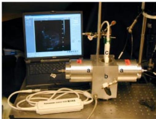
Fig. 1. View of pressure vessel after decompression and with the imaging probe in place. Diametrically opposed transducers (a) are used to generate (near-field) pressure levels up to 400 kPa in the vessel (b). Bubbles are viewed with diagnostic imaging (c), or a video camera (not shown).
