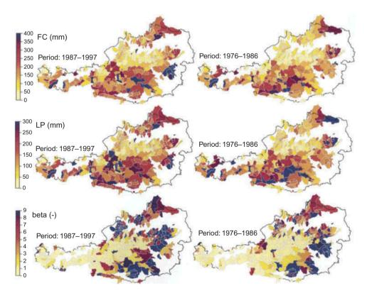
**Fig. 9** Spatial patterns of selected calibrated model parameters—top: maximum soil moisture storage FC (mm); centre: potential evaporation limit LP (mm); and bottom: nonlinearity parameter  $\beta$  (-)—for the calibration periods 1987–1997 (left) and 1976–1986 (right) (from Merz and Blöschl 2004, © 2004 Elsevier). This illustrates the potential of using spatial proximity as a proxy for functional proximity in densely gauged regions.
