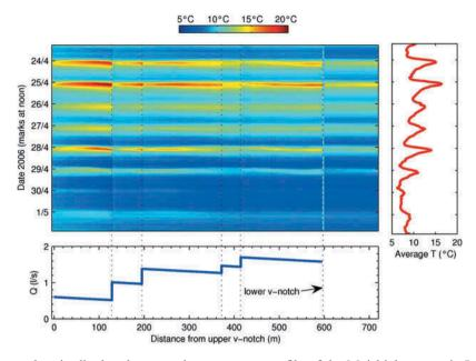
**Fig. 3** Observed continuous longitudinal and temporal temperature profile of the Maisbich stream in Luxembourg between 24 April and 1 May 2006. Clear temperature jumps can be seen at the location of the groundwater inflows (from Selker *et al.* 2006a, © 2006 John Wiley and Sons).
