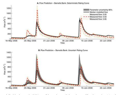
**Fig.** 7 Example of a modelled hydrograph (90% confidence interval) based on calibration using (a) a deterministic rating curve and (b) a rating curve including uncertainty (from McMillan *et al.* 2010,  $\bigcirc$  2010 John Wiley and Sons, Ltd.). This result illustrates the effect of rating curve uncertainty, which may add uncertainty to model predicitions, especially for estimating extremes.
