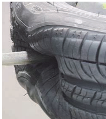
Figure: Tire deformation in breaking test.
