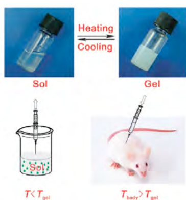
Figure 1: Schematic presentation of a thermogel with sol-gel transition upon heating.[3]
