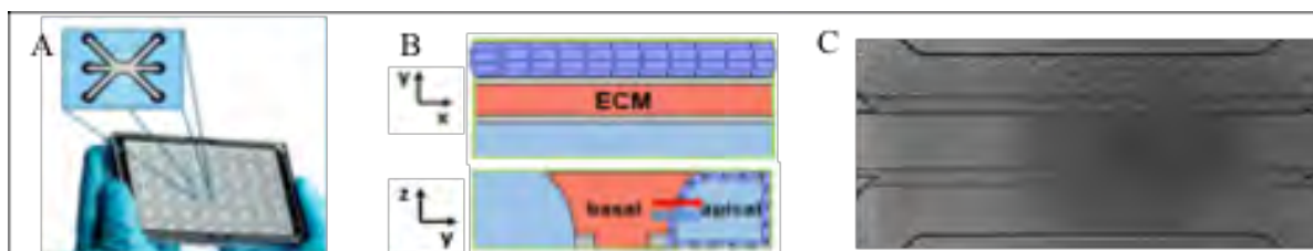
Figure 1: A) The 3-lane OrganoPlate ® platform with 40 microfluidic cell culture chips embedded in a standard 384-well microtiter plate. B) Schematic overview of RPTEC cells cultured against a collagen I ECM in a 3-lane OrganoPlate ® yielding access to both apical and basolateral side. C) Phase-contrast image of RPTEC cultured in the top channel of the OrganoPlate ® at day 7.
