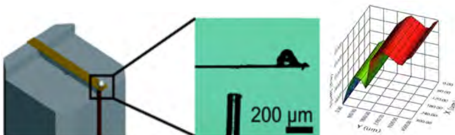
Figure 1: (left): Section of the measured grid showing an increase of E' over a length of 4.5mm. Figure 2: (right): Ferrule-top nanoindentation probe, including a cantilever and optical fiber for force readout [2].
