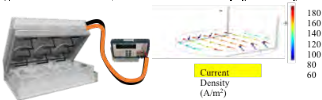
Figure 1: (left) Image demonstrating one of the direct electrode bioreactors; (right) steady state model of current density in in vitro set up.
