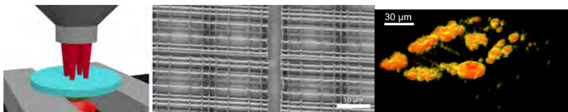
Figure 1: (left) Scheme of multi-foci laser direct writing. (middle) SEM of the 3D Nichoid micro scaffold fabricated using this technique. (right) 3D rendering of a coherent Raman image (CARS). Lipid vesicles showed an intense signal (2850 cm -1 ) and they are reconstructed from Z-stacks of MSCs cultured inside the Nichoid scaffold
