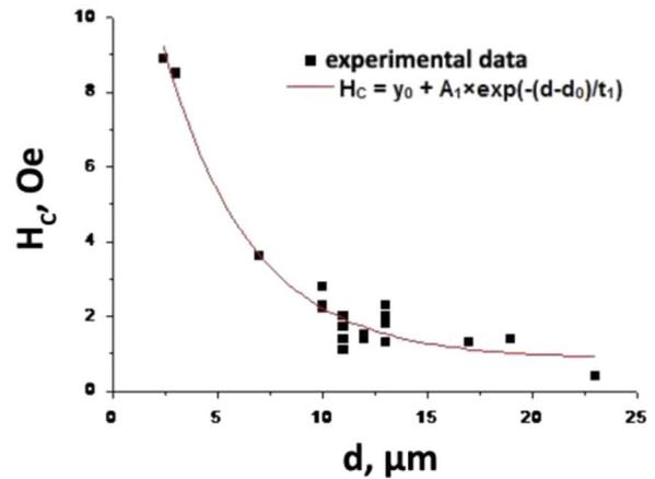
**Fig. 2.** The dependence of coercive force estimated from experimental data on diameter of the metallic nucleus of glass-coated microwires.
