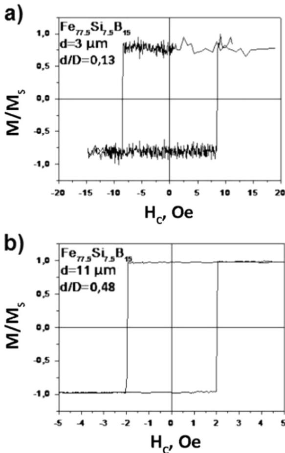
**Fig. 1.** The normalized hysteresis loops of the studied amorphous glass-coated microwires with different diameters of the nucleus and diameters ratio: (a)  $d = 3 \mu\text{m}$ ,  $d/D = 0.13$  and (b)  $d = 11 \mu\text{m}$  and  $d/D = 0.48$  ( $d$  – diameter of the metallic nucleus and  $D$  – total diameter of the microwire in the glass shell).
