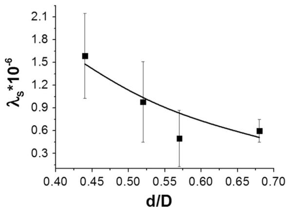
Fig. 6. Dependence of magnetostriction coefficient on the  $d/D$  for microwires with similar values of  $d \sim 12\text{--}13 \mu\text{m}$ .
