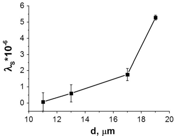
Fig. 5. Dependence of magnetostriction coefficient on the  $d$  for the microwires with similar values of  $d/D \sim 0.65\text{--}0.69$ .
