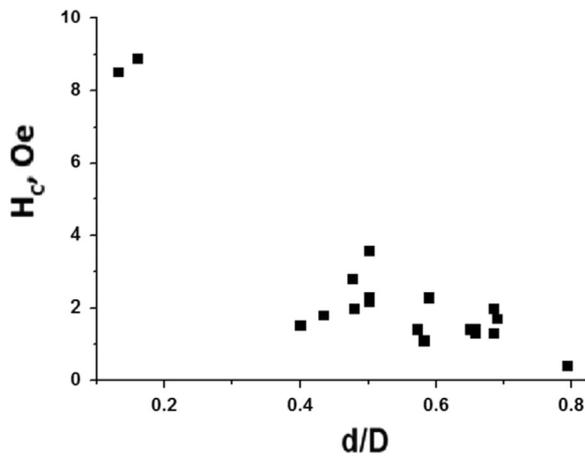
Fig. 3. The dependence of coercive force estimated from experimental data on  $d/D$ .
