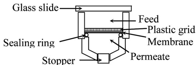
FIG. 1. Schematic diagram of the cell for diffusion experiments.
