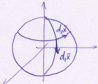
$$d\vec{S} = \frac{1}{2} \vec{e}_r \cdot 2 [\vec{e}_\theta R d\theta \times \vec{e}_\varphi R \sin \theta d\varphi] = R^2 \sin \theta d\theta d\varphi$$
