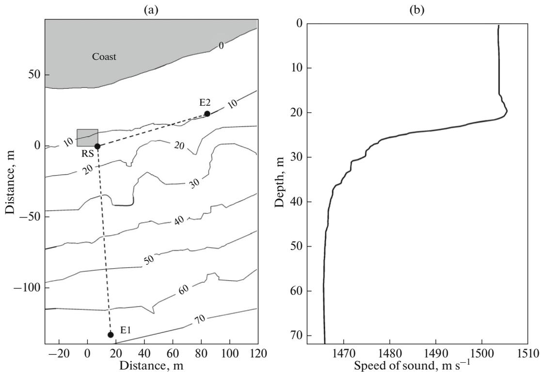
**Fig. 4.** (a) Bathymetric chart. RS is our three-element receiving system; E1 and E2 are the emitters. (b) Profile of the speed of sound.
