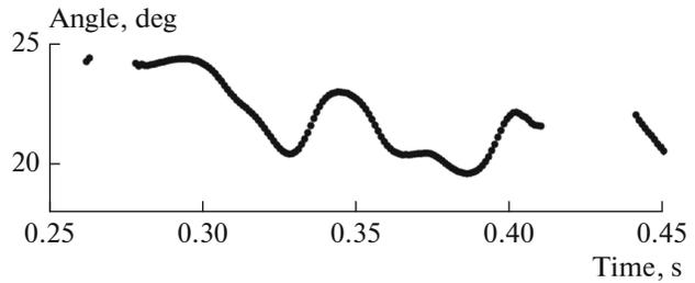
**Fig. 2.** Change in the angle of arrival for a pair of receivers of the seabed antenna (nos. 42 and 43).
