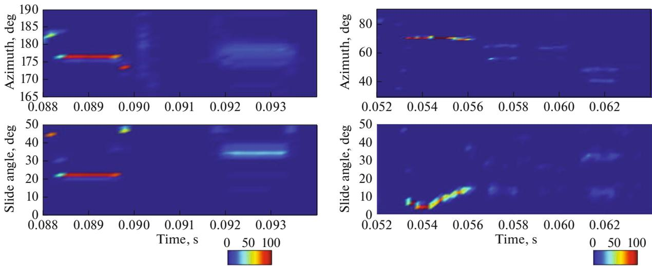
**Fig. 6.** Results from measuring the azimuths and slide angles for signals from sources E1 (left) and E2 (right). Color scales show the number of pulses out of 100 in a series falling in the interval of  $1^\circ$  in azimuth and  $2^\circ$  in the slide angle for the time of a given signal (time step, 0.00001 s).
