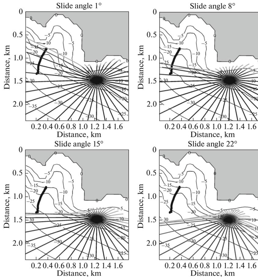
**Fig. 3.** Projections of ray paths on the horizontal plane with different slide angles. The transition from black to gray trajectories corresponds to the reduction in the intensity of sound.
