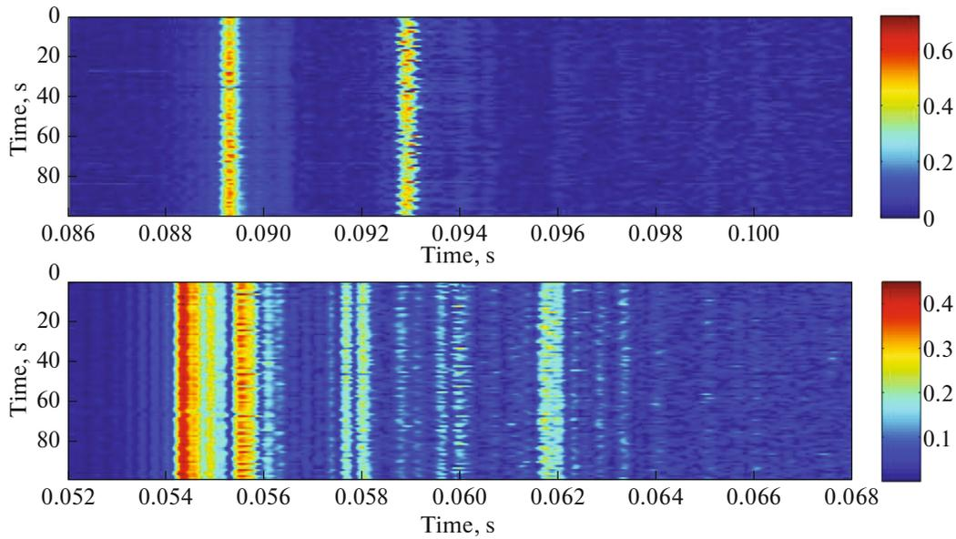
**Fig. 5.** Temporal variation of the envelope of cross-correlation function for received and emitted signals for E1 (top) and E2 (bottom). The time of emission is plotted along the ordinate axis; the time of signal arrival, along the abscissa axis. Colored scales show the values of the coefficient of cross correlation.
