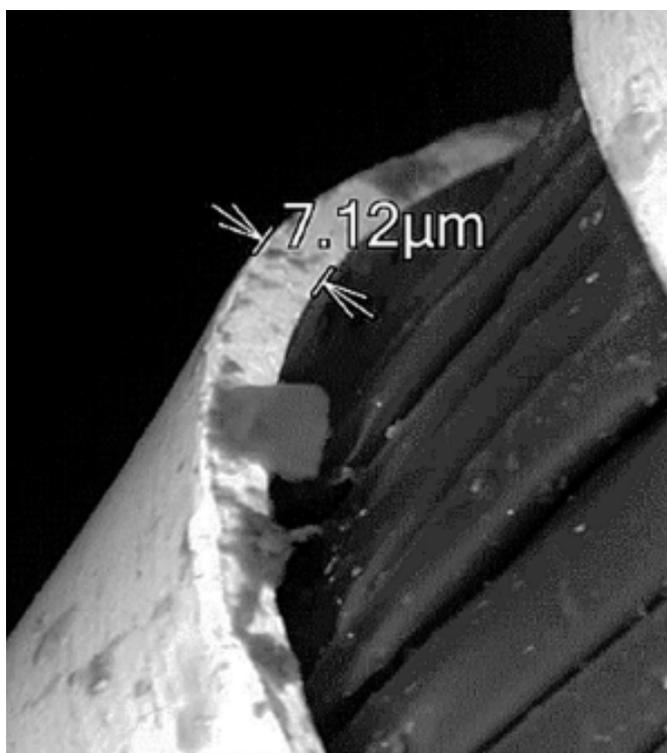
Figure 1: SEM photo of a metal thread.
