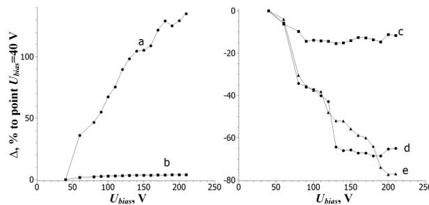
Figure 1: The y axis - the change in the value of the Si detector parameters (500  $\mu\text{m}$ , S - 90 mm<sup>2</sup>) as a percentage of the point with a bias voltage of 40 V. a- the signal amplitude in the slow channel, b- the amplitude in the fast channel, c- is the amplitude resolution, d- time resolution, e- the fast signal front at the level of 0.1-0.9.
