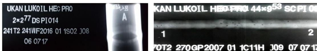
Figure 1: X-ray picture of welded seam sample (∅=50.8 mm) received by ionizing radiation source of Ir-192.
