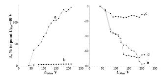
Figure 1: The y axis - the change in the value of the Si detector parameters (500  $\mu$ m, S - 90 mm<sup>2</sup>) as a percentage of the point with a bias voltage of 40 V. a- the signal amplitude in the slow channel, b- the amplitude in the fast channel, c- is the amplitude resolution, d- time resolution, e- the fast signal front at the level of 0.1-0.9.
