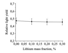
Figure 1: The dependence of the light yield of scintillators based on a copolymer of styrene and methacrylic acid containing 4% PPO, 0.02% POPOP and 15% naphthalene on the concentration of lithium (relatively to the light yield of unloaded polystyrene based plastic scintillator).
