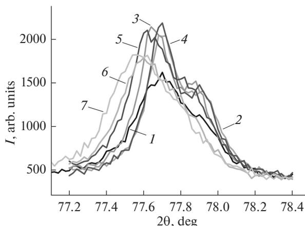
**Fig. 2.** Plots of diffraction patterns of the surface of ceramic samples  $[(\text{Na}_{0.5}\text{Bi}_{0.5})_{1-x}\text{K}_x]\text{TiO}_3$  from  $x = 0$  (1), 0.01 (2), 0.02 (3), 0.03 (4), 0.04 (5), 0.05 (6), 0.06 (7) obtained for  $T_1 = 1073$  K (6 h),  $T_2 = 1423$  K (2 h).
