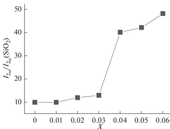
Fig. 4. Concentration dependence of the SHG signal intensity  $q = I_{2\omega}/I_{2\omega}(\text{SiO}_2)$  samples  $[(\text{Na}_{0.5}\text{Bi}_{0.5})_{1-x}\text{K}_x]\text{TiO}_3$  obtained for  $T_1 = 1073\ \text{K}$  (6 h),  $T_2 = 1423\ \text{K}$  (2 h).
