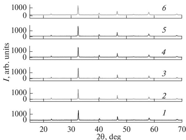
**Fig. 1.** Diffraction patterns of the surface of ceramic samples  $[(\text{Na}_{0.5}\text{Bi}_{0.5})_{1-x}\text{K}_x]\text{TiO}_3$  from  $x = 0$  (1), 0.01 (2), 0.02 (3), 0.03 (4), 0.04 (5), 0.05 (6), 0.06 (7) obtained for  $T_1 = 1073$  K (6 h),  $T_2 = 1423$  K (2 h).
