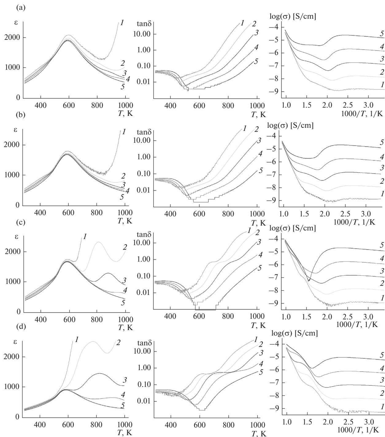
**Fig. 5.** Temperature dependences of the dielectric constant  $\epsilon$ , dielectric loss  $\tan\delta$  and electrical conductivity  $\log\sigma$  of the ceramic samples  $[(\text{Na}_{0.5}\text{Bi}_{0.5})_{1-x}\text{K}_x]\text{TiO}_3$  with  $x = 0.03$  (a),  $0.04$  (b),  $0.05$  (c),  $0.06$  (d), measured at frequencies of:  $f$ : 100 Hz (1); 1 kHz (2); 10 kHz (3); 100 kHz (4); 1 MHz (5).
