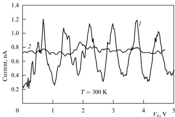
**Figure 4.** Curve (1): the dependence of the current through the molecular single-electron transistor on the gate voltage (dc bias point is shown by the arrow in Fig. 3). Curve (2): similar dependence when the STM tip is positioned above the stearic acid (without a cluster).
