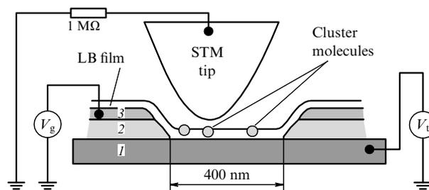
Figure 2. Schematic of the single-electron transistor based on a single cluster molecule. (1) HOPG substrate, (2) insulating layer ( $\text{Al}_2\text{O}_3$ ), (3) gold gate electrode.
