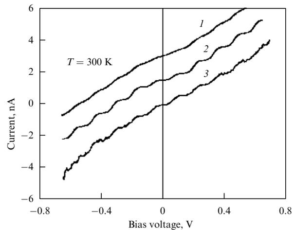
**Figure 5.**  $I$ - $V$  curves calculated using the 'orthodox' theory (curves 1 and 2) to fit the experimental result (curve 3). The curves are shifted vertically for clarity.
