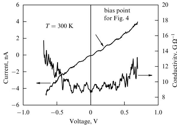
**Figure 3.** Typical  $I$ - $V$  curve and the differential conductance (as a function of bias voltage  $V$ ) for the molecular single-electron transistor.
