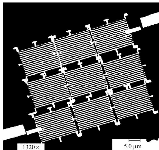
Figure 1. SEM image of the gate electrode fabricated before the monolayer deposition.
