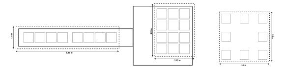
**Figure 1**. The area of interast (dashed line) of surface and underground counters of Tunka-Grande (left). The area of interest of Taiga-Muon (right).
