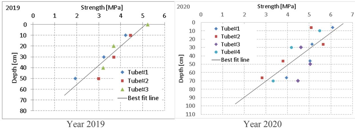
**Figure 7.** Distribution of uniaxial compressive strength of ice over its thickness as per the test data for thermally balanced samples
