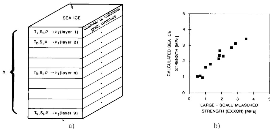
**Figure 1.** a) Ice fragmentation by layers over thickness, and b) comparison of ice compressive strength obtained with small samples using formula (2) and measured during full-scale tests (from Timko and Frederking, 1990)
