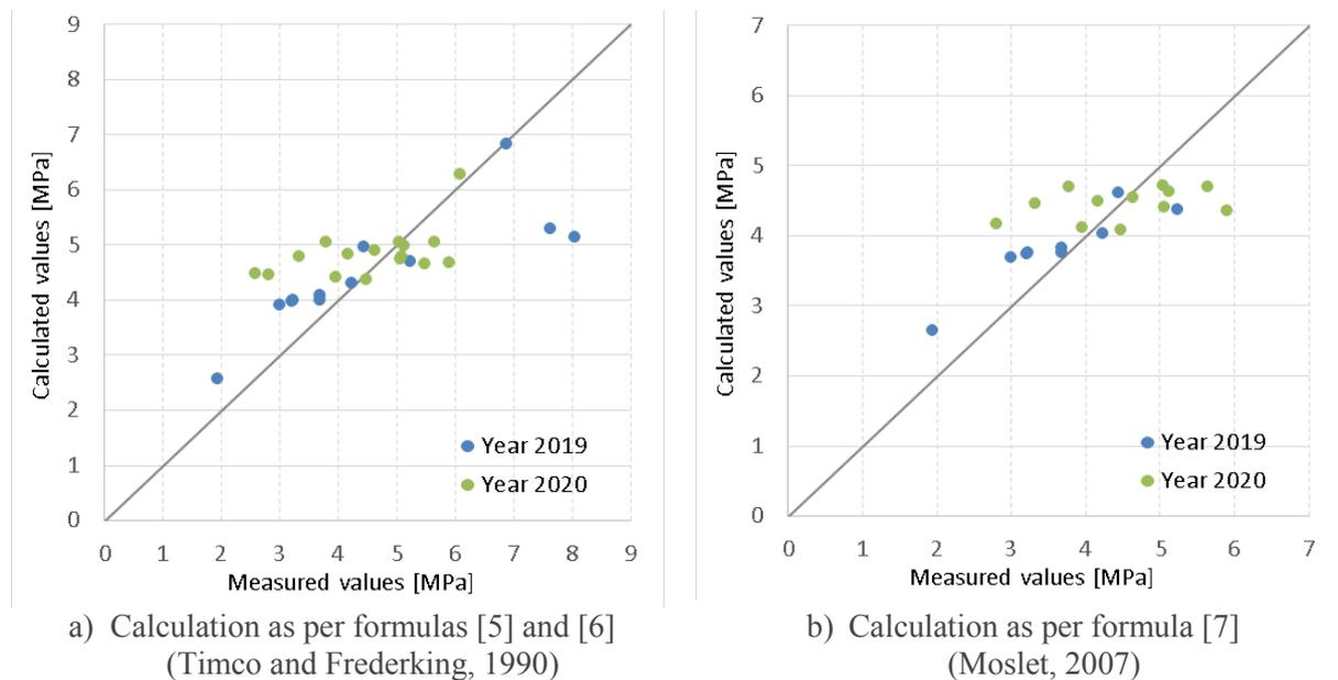
**Figure 8.** Comparison of small-tests results and calculations based on ISO 19906
