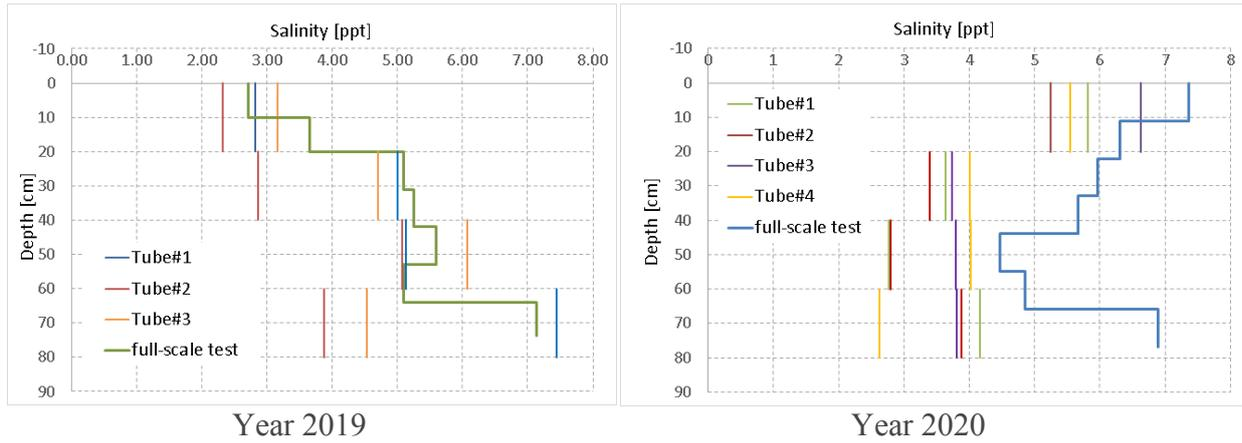
**Figure 6.** Salinity profiles over ice thickness, as measured on small ice samples and on ice cores drilled from ice cover next to full-scale tests
