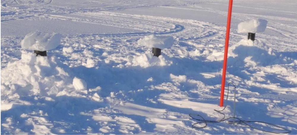
**Figure 3.** Workplace with tubes frozen into the ice cover. Next to the red stick is a thermistor string
