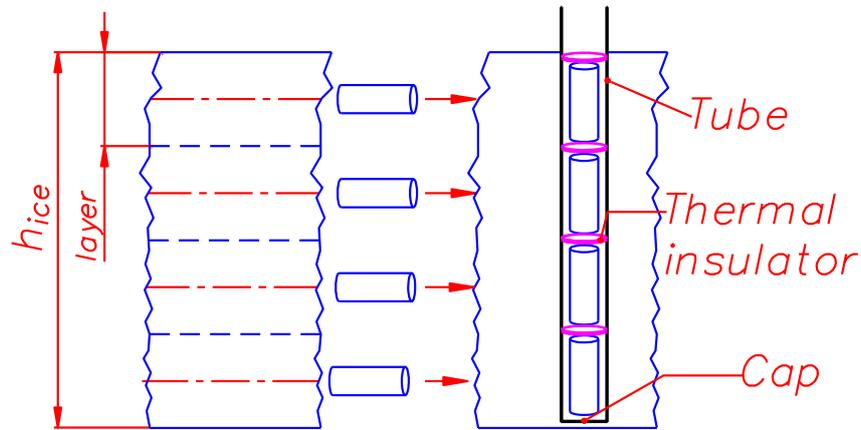
**Figure 2.** Preparation of thermally balanced ice samples
