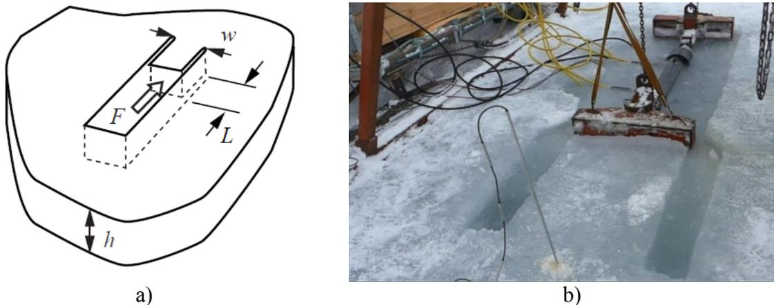
**Figure 4.** Full-scale compression test: a) layout, and b) set-up
