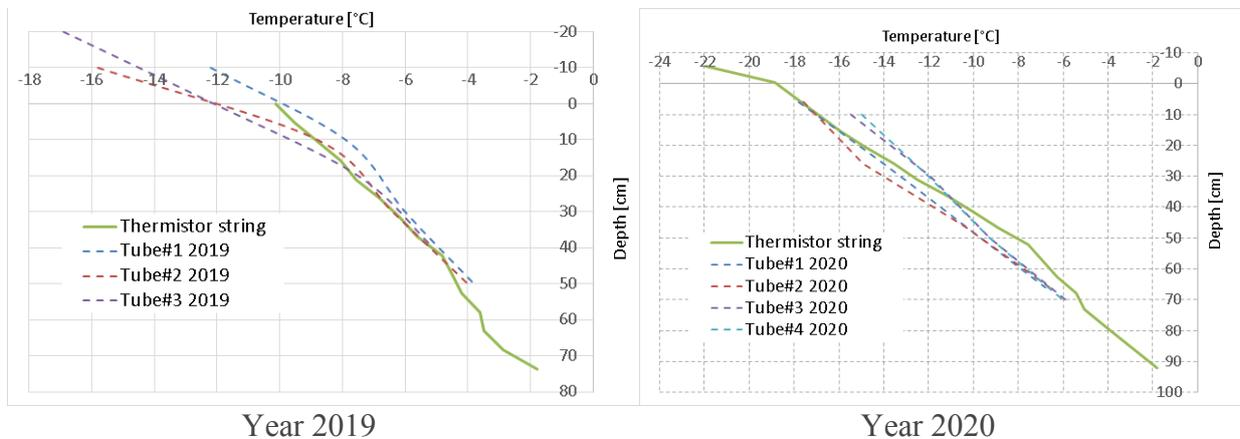
**Figure 5.** Temperature profiles over ice thickness, as measured on small ice samples and in ice cover using a thermistor string
