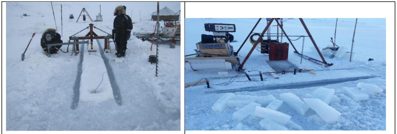
Figure 6. Setup for a field test (frames to apply load and to measure deflection and pressure): (a) FEB test (vertical load), and (b) FEB test (horizontal load) with pressure sensors GEOKON (2018-03-08).
