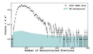
FIG. 7. Spectrum of events selected in triple coincidence (black), compared with accidentals with  $f_{90} < 0.4$  from the UAr sample, normalized to events selected in the AmBe sample with  $N_e$  in the [200, 500] range.
