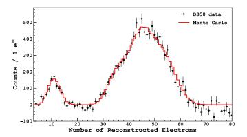
FIG. 1. Comparison between the best-fitted simulated spectrum and <sup>37</sup>Ar data as a function of the reconstructed number of electrons. The free parameters in the model are the mean number of ionization electrons induced by the <sup>37</sup>Ar L1- and K-shell electrons, and the Fano factor.
