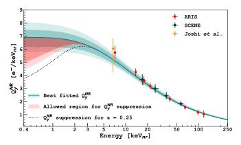
FIG. 11. Allowed region (red) for low energy  $Q_y^{\rm NR}$  suppression tested on the AmC dataset, and best-fitted  $Q_y^{\rm NR}$  (blue), using the Ziegler *et al.* screening function. Dark (light) shaded area corresponds to  $1\sigma$  ( $2\sigma$ ) uncertainty. The dashed line represents the  $Q_y^{\rm NR}$  suppression tested in [36] assuming Eq. (16) with z=0.25.
