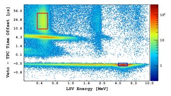
FIG. 6. Veto selection of prompt (blue box) and delayed (red box) events associated to AmBe neutron emission, as a function of liquid scintillator veto (LSV) visible energy and time difference between veto and TPC signals. The trigger time offset between the two detectors is about -550 ns. The horizontal feature at the 4.3  $\mu$ s offset is due to PMT afterpulses.
