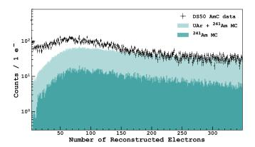
FIG. 4. Comparison between AmC spectrum (black) and contamination from TPC intrinsic events and  $\gamma$ s from <sup>241</sup>Am, as described in the text. The low-energy excess is due nuclear recoils induced by neutrons.
