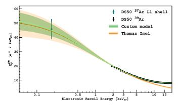
FIG. 2. Fit of the ER ionization yield, measured from AAr (black) and  $^{37}$ Ar (teal) data with a drift field of 200 V/cm, with the Thomas-Imel box model up to 3 keV<sub>er</sub> [Eq. (4)], and with the custom model from Eq. (6), which extends the Thomas-Imel model up to 20 keV<sub>er</sub>. The model bands correspond to  $1\sigma$ , also accounting for the correlation from the  $g_2$  systematics, which dominates the experimental uncertainties.
