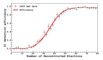
FIG. 5. Efficiency in detecting S1 + S2 events  $(N_{2p})$  with respect to S1 + S2 and S2 only  $(N_{1p})$ , as a function of the reconstructed number of electrons. Data are fitted with an error function (red line). The error band is propagated from the uncertainties of the fitted parameters.
