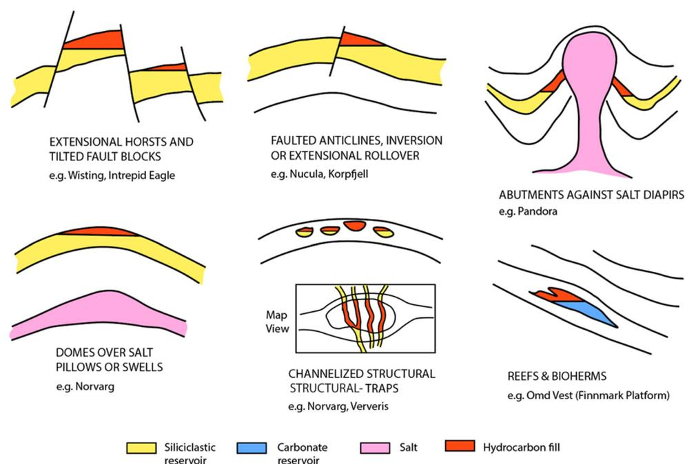
**Fig. 17.** Schematic sketches of the principal trapping styles, proven and postulated, with example discoveries in the South-Central Barents Sea Composite TSE.
