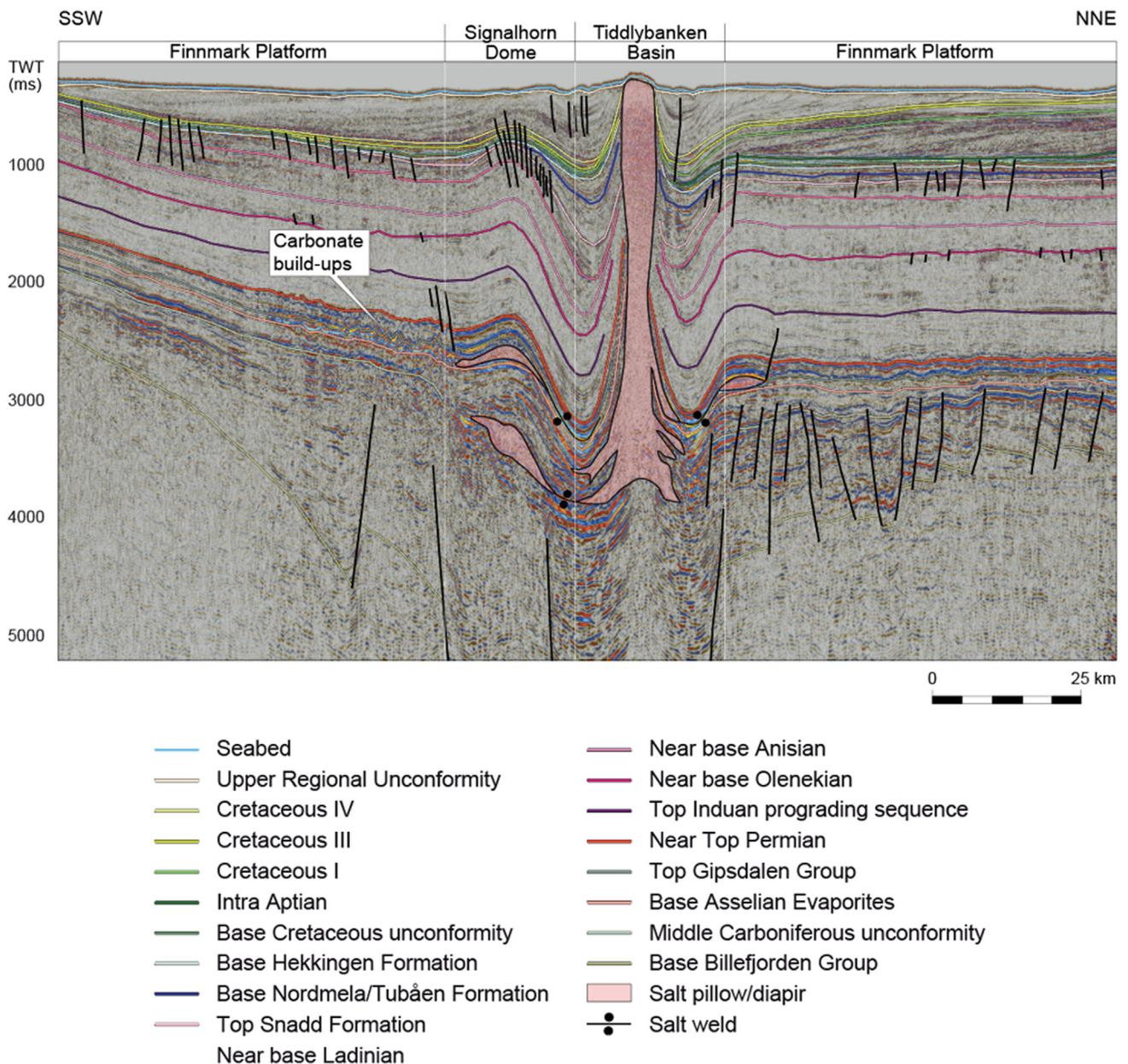
**Fig. 11.** NE–SW seismic line over the Tiddlybanken Basin (line E in Fig. 3) showing late Paleozoic basinal structure, salt withdrawal and multi-phase halokinesis. The recently drilled Signalhorn Dome and carbonate organic build-ups in the Permian interval are also clearly shown. The seismic line is shown courtesy of the Norwegian Petroleum Directorate (NPD).
