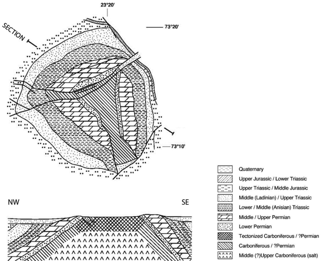
**Fig. 12.** Subcrop map and cross-section over the salt-induced Svalis Dome in the west of the TSE (line F in Fig. 3). Late movement on the structure has brought Triassic and late Paleozoic successions to shallow depth, and, hence, has provided a critical sampling point in the south-central Barents Sea. Figure adapted from Hochuli and Feist-Burkhardt (2004).
