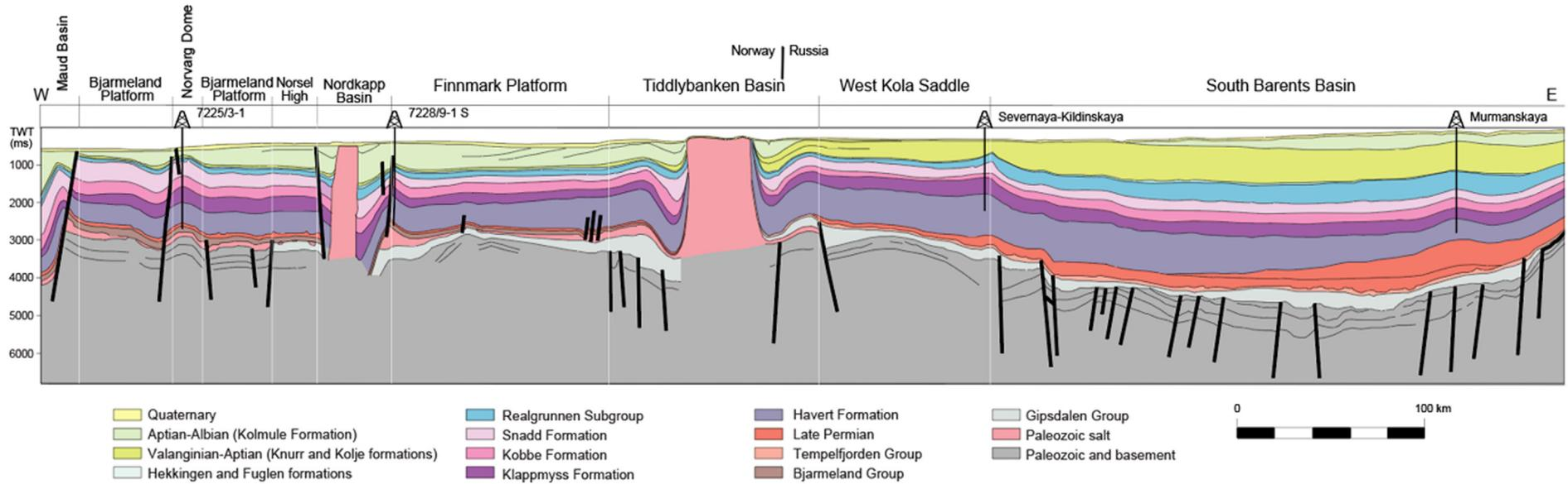
**Fig. 7.** West-east super-regional geoseismic profile (line A in Fig. 3) crossing the Bjarmeland Platform, Nordkapp Basin, Finnmark Platform, Tiddlybanken Basin and South Barents Basin.
