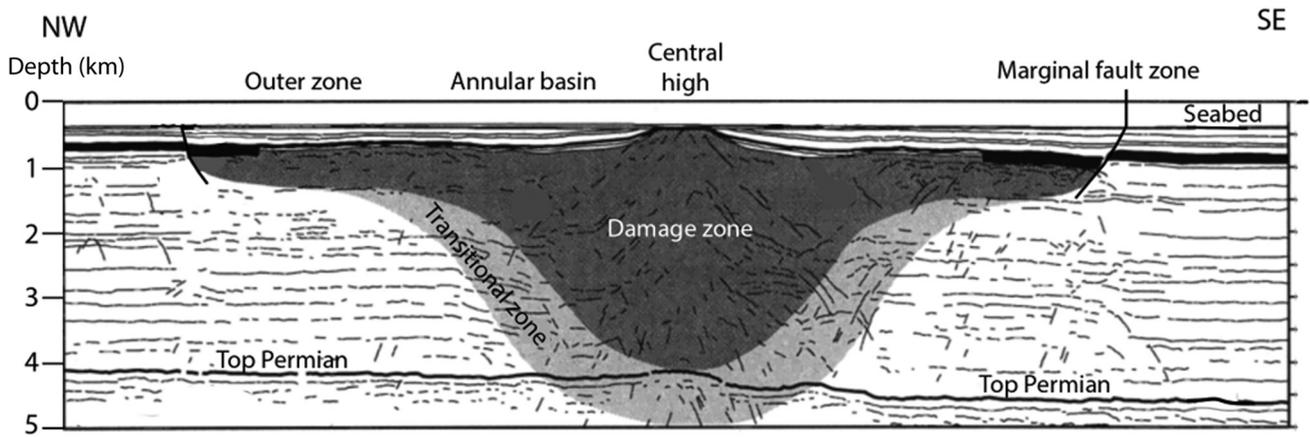
**Fig. 14.** Geoseismic profile over the Mjølner impact structure (line H in Fig. 3). Figure adapted from Tsikalas (1996).
