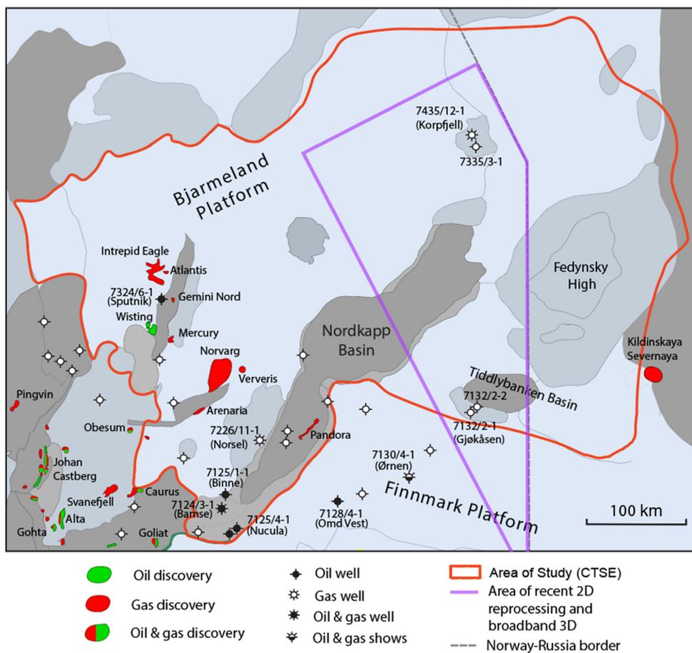
**Fig. 2.** Location of discoveries and selected wells described in this paper. Where the outlines of discoveries are indicated, discovery and appraisal wells are not shown. The purple outline shows the area of intensive 2D seismic reprocessing and 3D broadband seismic acquisition, associated with the Norwegian 23rd Licensing Round. Structural elements from Figure 3 are shown in greyscale for reference.
