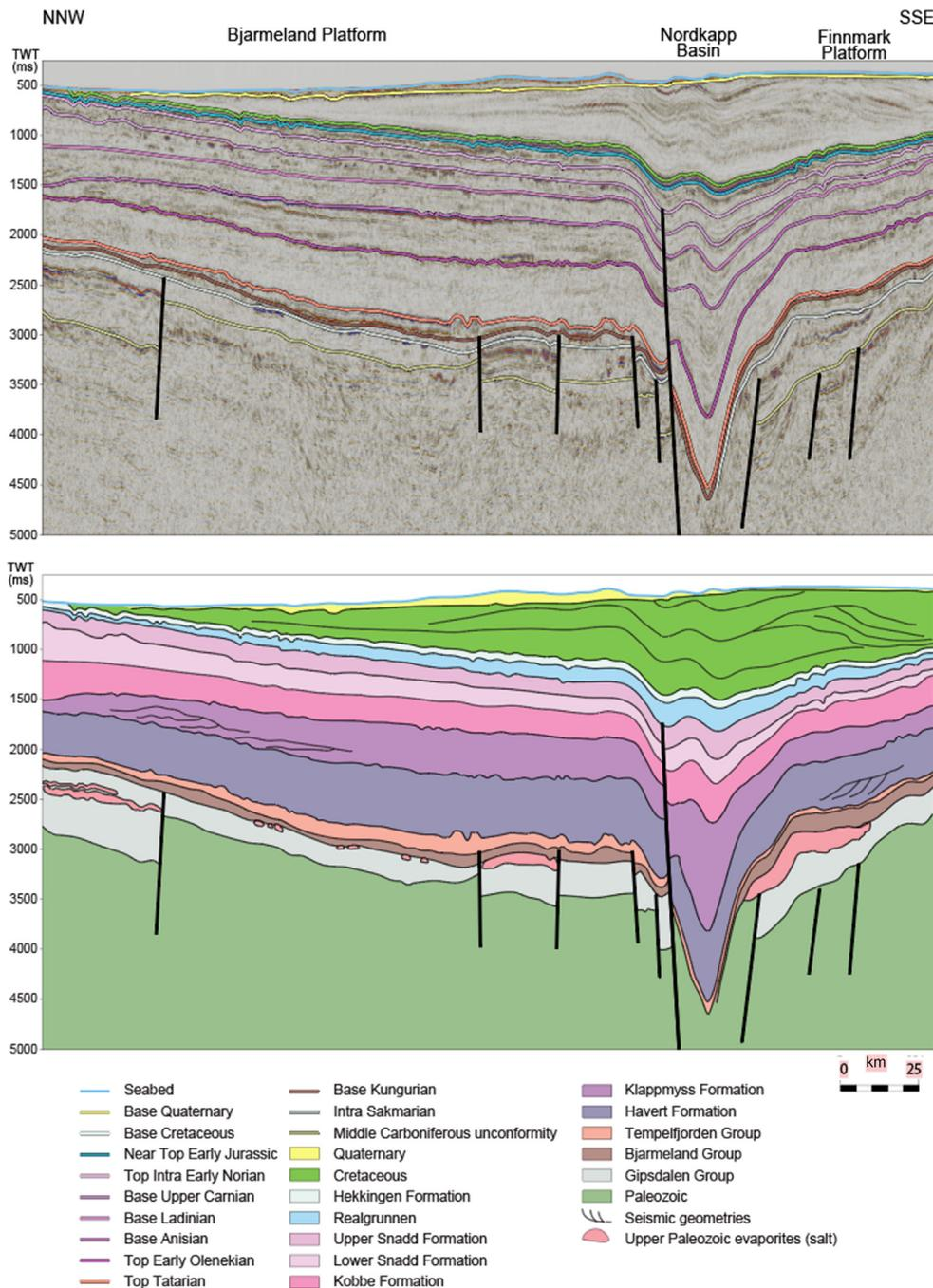
**Fig. 10.** North-south interpreted seismic line and geoseismic profile (line D in Fig. 3) over the Bjarmeland Platform, Nordkapp Basin and Finnmark Platform. The seismic line is shown courtesy of TGS.
