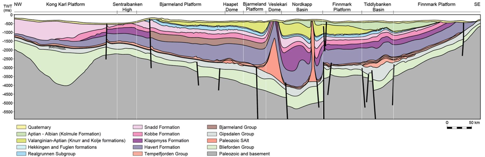
**Fig. 9.** NW-SE super-regional geoseismic profile (line C in Fig. 3) crossing the Kong Karl Platform, Bjarmeland Platform, Haapet Dome, Nordkapp Basin and Finnmark Platform.
