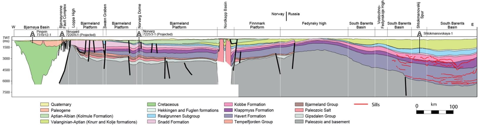
**Fig. 8.** West-east super-regional geoseismic profile (line B in Fig. 3) crossing the Bjarmeland Platform, Nordkapp Basin, Finnmark Platform, Fedynsky High and South Barents Sea Basin.
