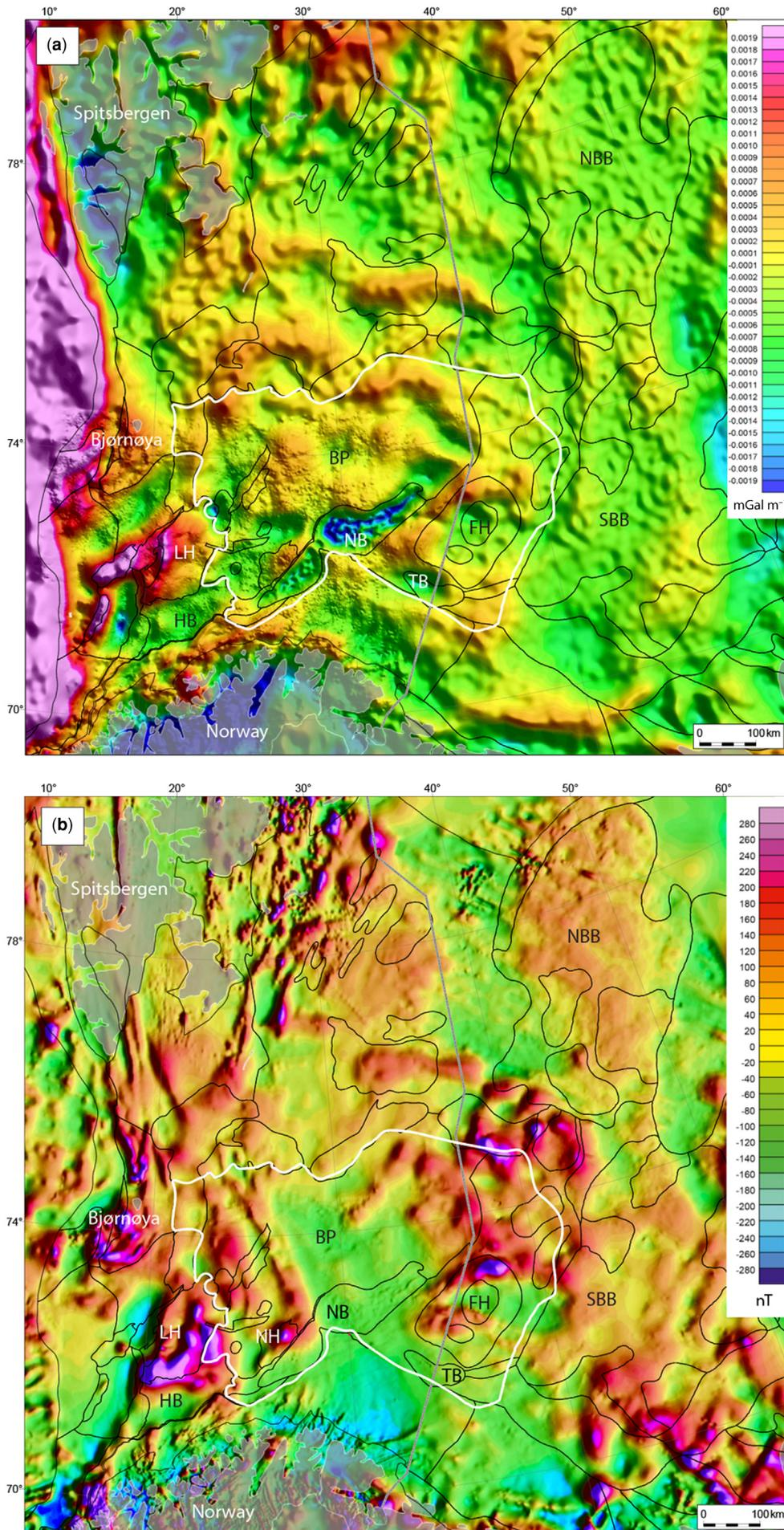
**Fig. 6.** Gravity and magnetic maps of the Barents Sea, showing the TSE location and setting. (a) Bouguer gravity map. (b) Total intensity magnetic map. Basin outlines are shown for reference. Abbreviations: BP, Bjarmeland Platform; HB, Hammerfest Basin; FH, Fedynsky High; LH, Loppa High; NB, Nordkapp Basin; SBB, South Barents Basin; TB, Tiddlybanken Basin.
