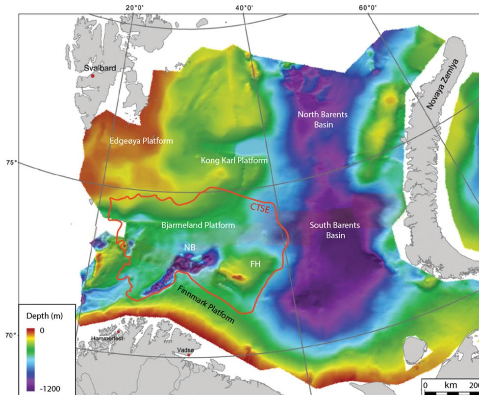
**Fig. 15.** Near Base Permian depth map of the Barents Sea, illustrating the sediment thickness distribution in and adjacent to the South-Central Barents Sea CTSE. Abbreviations: FH, Fedynsky High; NB, Nordkapp Basin. Modified after Henriksen *et al.* (2011b).
