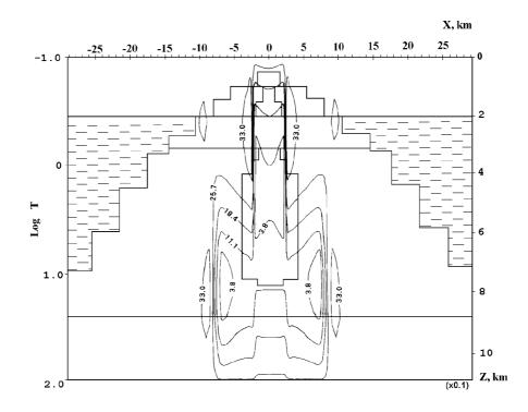
**Fig. 2**.  $\phi_{xy}$  (×10<sup>-1</sup>) pseudo-section for volcano model shown in Fig. 1.
