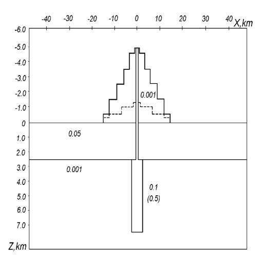
**Fig. 8**. Geoelectric model of a typical volcano (vertical cross-section under the central profile). The figures show electrical conductivity values in S/m.
