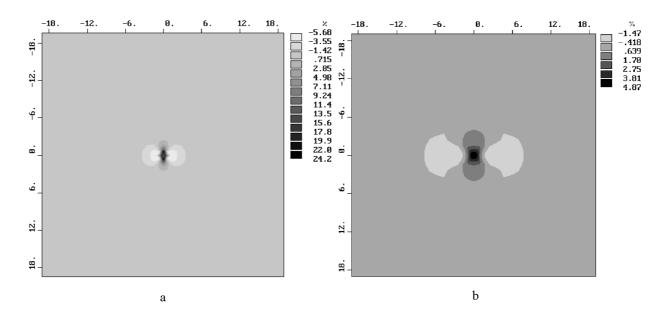
**Fig. 10a,b.** Isolines of normalized amplitude differences (in %) of the component  $H_x$  at a period T = 1 s: *a*) - in the case of the cone absence and b) - at its presence.
