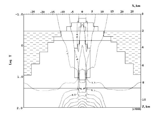
**Fig. 4**. *Re*  $Z_{vx}$  (×10<sup>2</sup>) pseudo-section for volcano model shown in Fig. 1.
