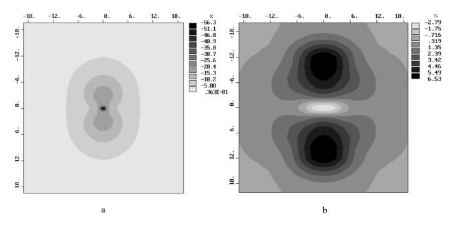
**Fig. 12.** Maps of difference isolines (in %) of normalized amplitudes of electric field component  $E_y$  at the period T=10 s: a) in the case of the cone absence, b) at its presence.
