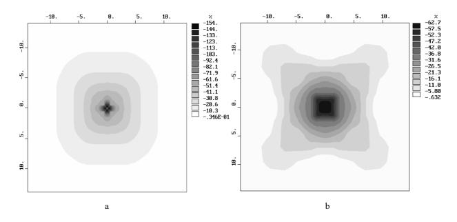
**Fig. 13a,b.** Map of difference isolines (in %) of normalized values  $\rho_{det}$  at the period T=10 s a) in the case of the cone absence and b) at its presence.
