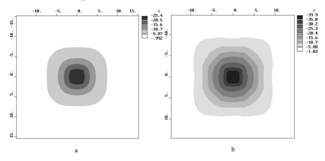
**Fig. 14a,b.** Map of differences isolines (in %) of normalized values  $\rho_{det}$  at the period T = 10 s for the model without the magma channel shown in a Fig. 8 at decrease of resistivity in the magma chamber: a) in 2 times; b) in 5 times.
