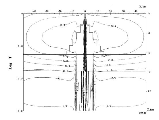
**Fig. 9.**  $\varphi_{xy}$  (×10<sup>-1</sup>) pseudo-section in *XOZ* plane.
