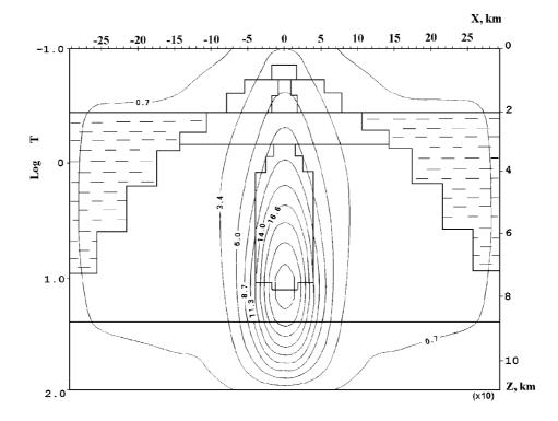
**Fig. 6.** Im  $E_y(\times 10^1)$  pseudo-section for volcano model shown in Fig.1. Result is based on an incident electric field, parallel to  $O_y$ -axis.
