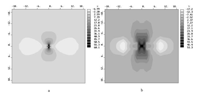
**Fig. 11a,b.** Maps of difference isolines (in %) of normalized amplitudes of magnetic field component  $H_x$  at the period T=10 s: a) in the case of the cone absence and b) at its presence.
