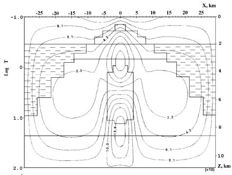
**Fig. 5**.  $ReE_y(\times 10^1)$  pseudo-section for volcano model shown in Fig.1. Result is based on an incident electric field, parallel to  $O_y$ -axis.
