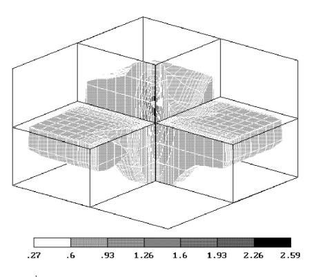
**Fig. 7. Im**  $E_{y}(\times 10^{1})$  iso-surfaces for volcano model shown in Fig.1.
