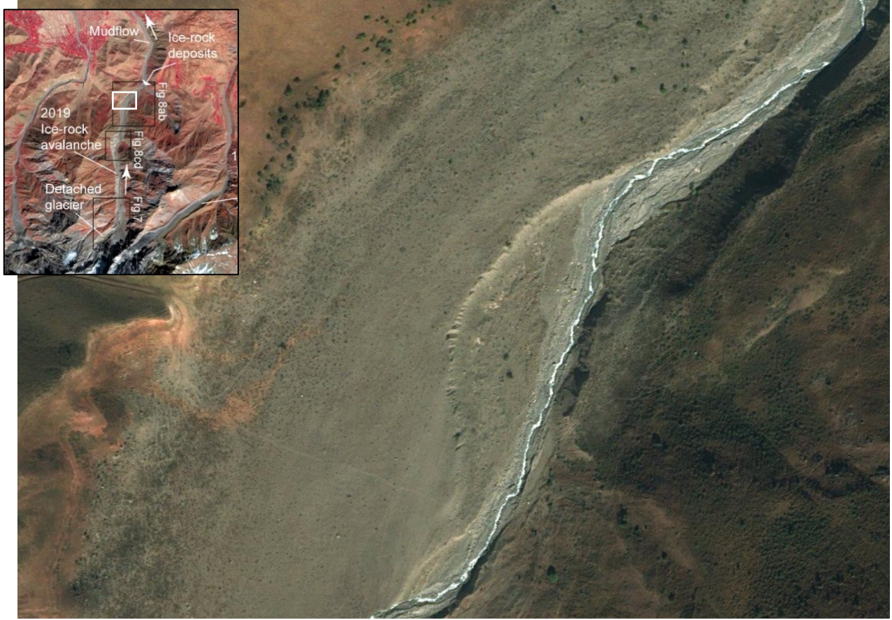
Fig. S4: Later deposit area of the Rasht 2019 detachment showing features of a potential earlier ice-rock avalanche (streamlined features to the middle and lower part; rough chaotic microtopography to the upper right). (© GoogleEarth, Maxar). Width of section: 0.7 km. North to the top. Position of image section indicated as white rectangle in the upper left inset.
