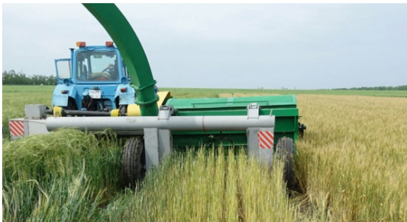
Fig. 1. Winter wheat harvesting with a trailed combing header loading unmilled grain heap into a vehicle
