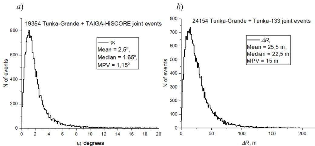
Fig. 2. The accuracy of the EAS arrival direction reconstruction by the Tunka-Grande array in comparison with data of TAIGA-HiSCORE array (a) and the accuracy of the EAS core position reconstruction by the Tunka-Grande array in comparison with data of Tunka-133 facility (b)
