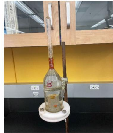
(b) Sample B 100% saturated with oil in Amott cell containing water – spontaneous displacement of oil by water clearly seen (a strongly water wet system)
