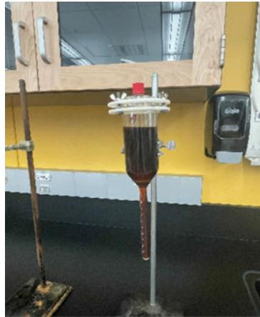
(a) Sample A 100% saturated with water in Amott cell containing Umiat oil – no spontaneous displacement of water by oil
