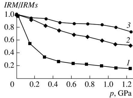
**Fig. 2.** Normalized isothermal remanent magnetization  $IRM/IRM_s$  vs. the applied pressure for the samples of (1) quartzitic microdiorite (magnetite), (2) alkali basalt (titanomagnetite), and (3) rhyolite pyroclastic (hematite).  $IRM_s$  is the saturation isothermal remanent magnetization.
