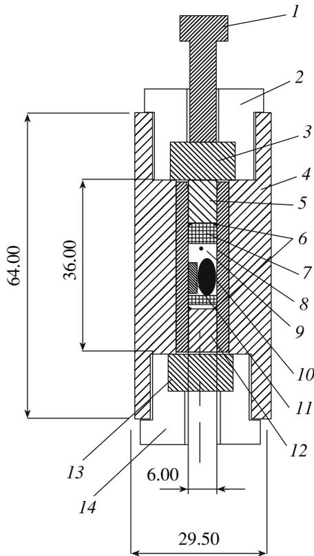
**Fig. 1.** Scheme of nonmagnetic high-pressure cell: (1) external piston, (2) upper retention screw, (3) bearing, (4) cell's body, (5) internal piston, (6) antiextrusion rings, (7) Teflon plug, (8) Teflon cavity, (9) pressure-transmitting fluid (PES-1), (10) sample, (11) Teflon spiral to keep sample fixed, (12) internal piston, (13) bearing, and (14) lower retention screw. The dimensions are given in mm.
