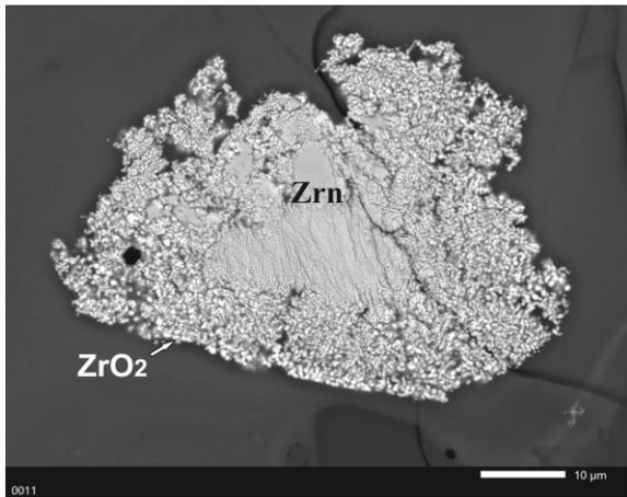
**Fig. 1** Rim of granular textures in zircon with dissociation of zircon into  $ZrO_2$  and  $SiO_2$
