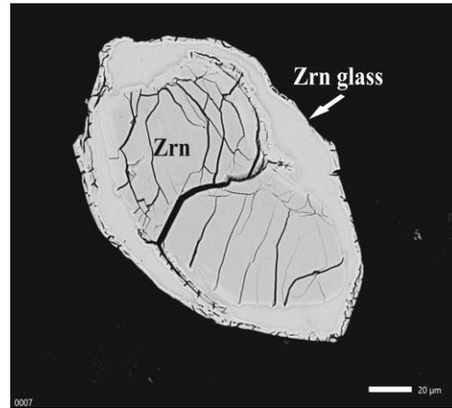
**Fig. 2.** Rim of fused zircon glass from the suevite of the Logoisk structure
