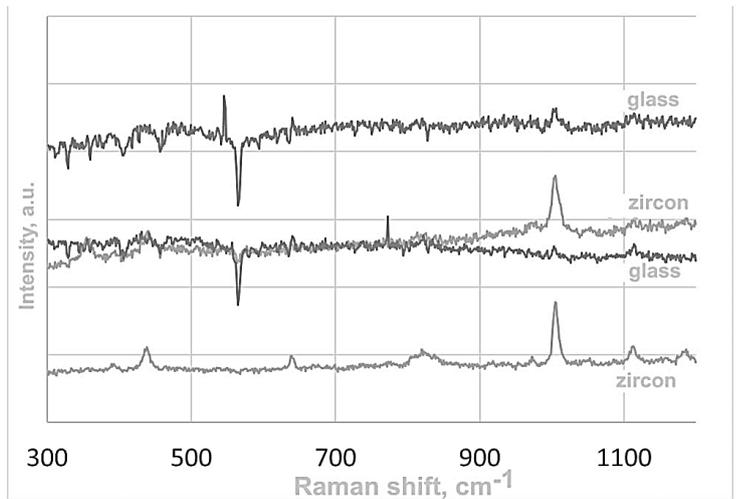
**Fig. 4.** Raman spectroscopy in zircon (grey lines) and diaplectic glass (dark lines) from Logoisk structure.
