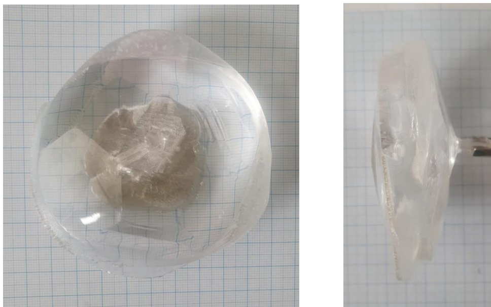
Fig. 1. BBO crystal weighted 422g, top and side views.
