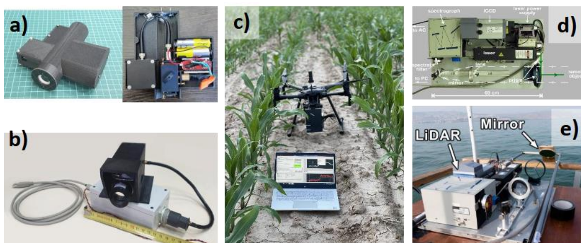
Fig. 1. Compact fluorescence (a) and eye-safe (b) LIDAR systems developed at Prokhorov General Physics Institute of RAS. Compact LIDAR installed at a small drone (c). Raman LIDAR (d) developed for fresh and seawater monitoring (e).
