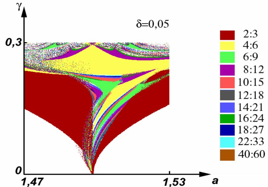
Phase diagram for sine mapping of a circle taking into account the refractory period (6) and stable phase captures of the sine mapping (6) inside the 2:3 capture splitting region.
