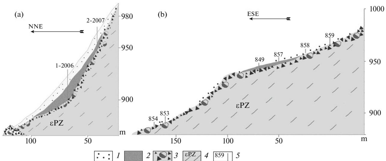
**Fig. 5.** The internal structure of glacier (a) no. 2 and (b) no. 3 based on the results of pitting and drilling in 2006–2007: ice (1), snow (2), crushed stone and lumps (3), alkaline rocks (4), and numbers of boreholes (5).
