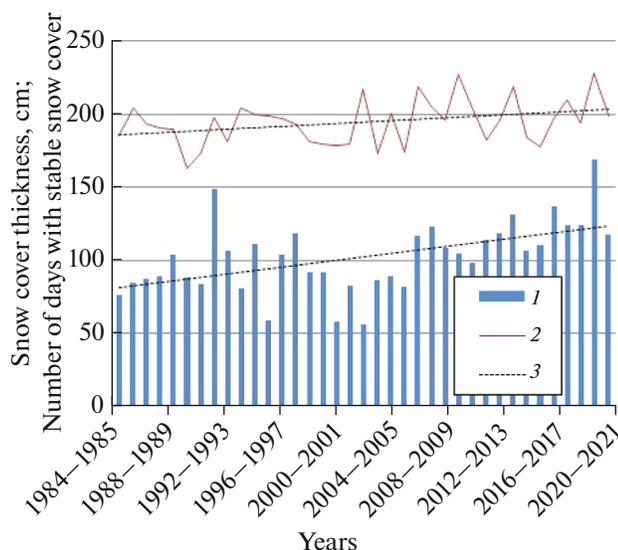
**Fig. 4.** Variations in the maximum snow cover thickness and the duration of stable snow period at the meteorological site of the Khibiny Educational and Scientific Station: snow cover thickness (1), number of days with stable snow cover (2), and trend lines (3).
