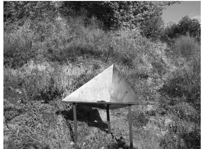
Fig. 2. The corner reflector installed in the lower part of the landslide slope near Mamaika village.
