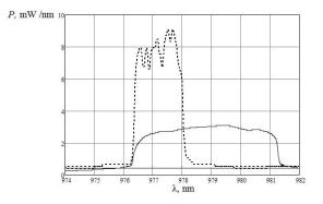
**Fig. 2.** Spectral characteristics of the KLM980-5-15 diode, measured at the beginning of the work (dotted curve), and after a year of operation (solid curve).
