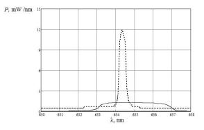
**Fig. 1.** Spectral characteristics of the KLM-D650-5-5 diode, measured at the beginning of the work (dotted curve), and after a year of operation (solid curve).
